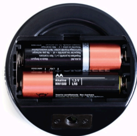
▲ Figure 5.7 When one coulomb of charge passes through both these cells in turn it gains 3 J of energy.
