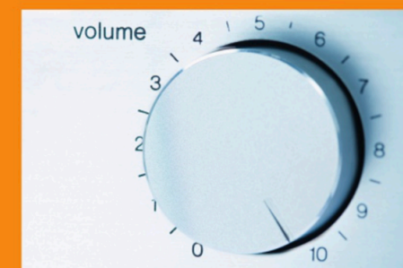
▲ Figure 6.1 Turning this dial alters the resistance in the circuit which changes the volume of the sound.
