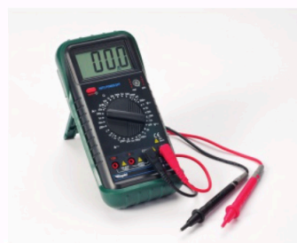
▲ Figure 5.3 An ammeter is used to measure current in a circuit. It has a very low resistance and so has almost no effect on the current.
