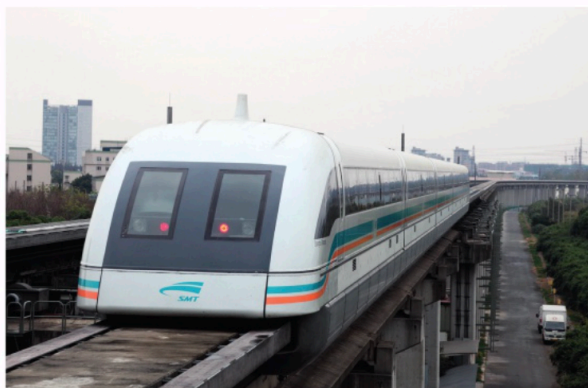
▲ Figure 6.20 Maglev trains use superconducting magnets to help them hover above the tracks.
