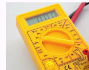
▲ Figure 5.8 A voltmeter measures voltages across a component.
