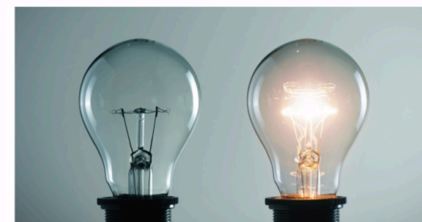
▲ Figure 4.11 It is the heating effect of a current that is causing this bulb to glow.
