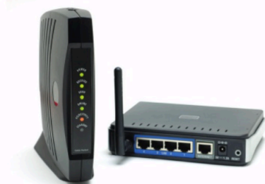
▲ Figure 5.11 Glowing LEDs indicate which circuits are working
