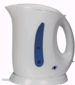
▲ Figure 4.8 This plastic kettle has double insulation which means that there is no need for an earth wire.
