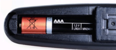
▲ Figure 5.6 When one coulomb of charge passes through this cell it gains 1.5 J of energy.
