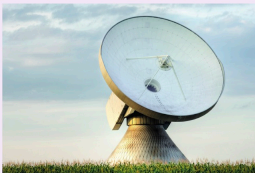
▲ Figure 7.16 Radio telescopes have concave reflecting dishes so that the signals from space reflect and converge onto a detector that is placed in front of the dish.
